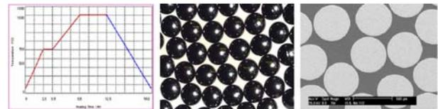
Fig.5. Sintering mode and  $\text{UO}_2$  particles.
